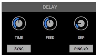
The main delay line. Input first goes through it and the processed feedback is sent back to it.
