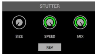
This effect is the first in the feedback signal chain. It loops short slices of the incoming audio which can then be played back at a different speeds and backwards.
