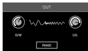
**D/W** : a standard dry/wet mix knob allowing you to blend the amount of the effect with fully counter clockwise being zero effect, and fully clockwise being 100% effect.
