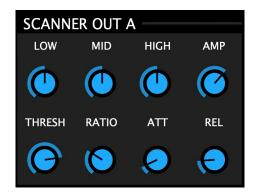
The Scanner Output module features a three band EQ and a utility compressor to help you sculpt the audio output of each scanner.
