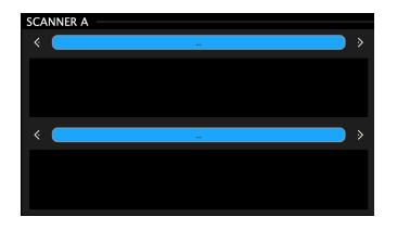
The Scanner modules feature two sample slots where you can load audio files included in the Factory Sample Bank or from your own collection.
