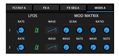
The MODS module offers 2 additional LFOs along with a modulation matrix. These LFOs allow you to build complex modulation layers on top of the Scan and Ratio LFOs.
