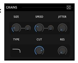
This module buffers its input into a delay line and several playheads loop small random sections of the delay line at the same time (grains).
