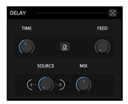
This module is a standard delay line with feedback control and adjustable mix. It features a variable input routing knob that allows you to either take input from the Buffer or Grains modules, or to blend the incoming signals as desired.
