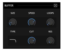
This module records a small portion of the input signal and loops it a certain number of times, as defined by the user. The module also features a dedicated multimode filter.
