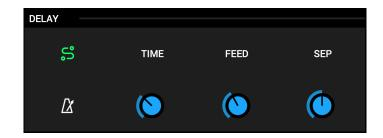
**TIME :** controls the delay time. The value can either be in milliseconds or in bar divisions if the «Sync» switch (metronome icon) is active. In sync mode, if the tempo goes below 40 BPM, the value displayed may be inaccurate as values exceeding the maximum delay size will be divided by 2. Range : 5Ms to 1000Ms in free mode, or 1 to 128 bar divisions in sync mode
