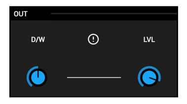
**D/W** : a standard dry/wet mix knob allowing you to blend the amount of the effect with fully counter clockwise being zero effect, and fully clockwise being 100% effect.
