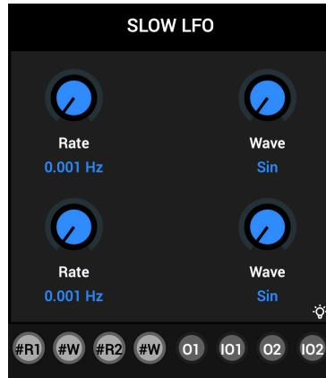
Two LFOs that are properly scaled for use as a modulation source. Each LFO outputs a regular and inverted signal and the Rate and Wave parameters can be modulated.
