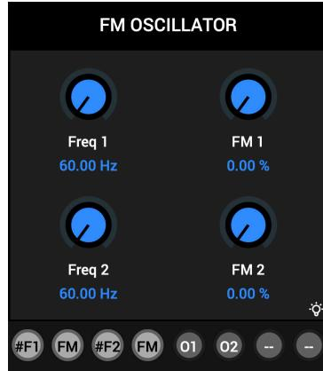
Two sinusoidal oscillators operating at audio range with Frequency Modulation inputs.
