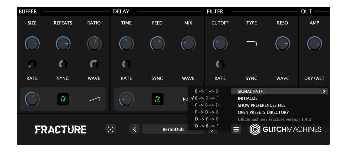
At Fracture's Configuration Menu (small gear icon in the footer) lies a drop down menu which allows you to reconfigure the order of the effects in the chain. This is extremely useful since the order of the effects significantly influences the sound of a given patch.
