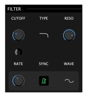
This module is a classic multi-mode filter which can act as a lowpass, highpass, bandpass or notch filter.
