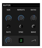
This module records a small portion of the input signal and loops it a certain number of times, as defined by the user. When it has finished looping, it automatically records the current input and starts looping again. The playback rate of the looped audio can be adjusted by the user.
