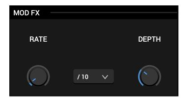
This effect is applied to the output of the filter but happens on the opposite audio channel. It's then routed back to the feedback input of the first delay on the original channel.
