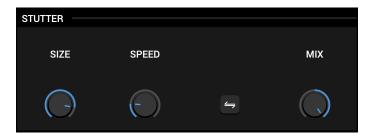
This effect is the first in the feedback signal chain. It loops short slices of the incoming audio which can then be played back at a different speeds and backwards.
