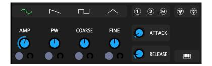
Waveform Select: click to select Sine, Sawtooth, Square or Triangle waveshapes
